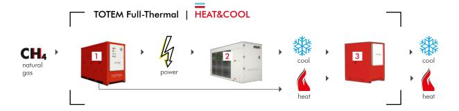
Choosing the TOTEM Full-Thermal means relying on the TOTEM micro-cogenerator benefits (efficient production of electricity and heat) as well as on the AERMEC heat pump high performances.
